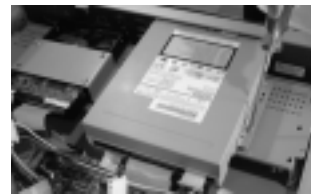
Fix the CD-RW with bolts on the bracket
